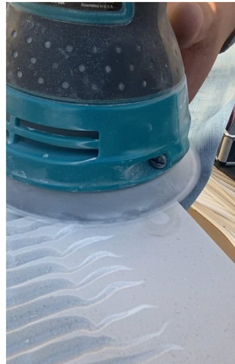
Step 3: Use a high grit sander to finish the surface.
